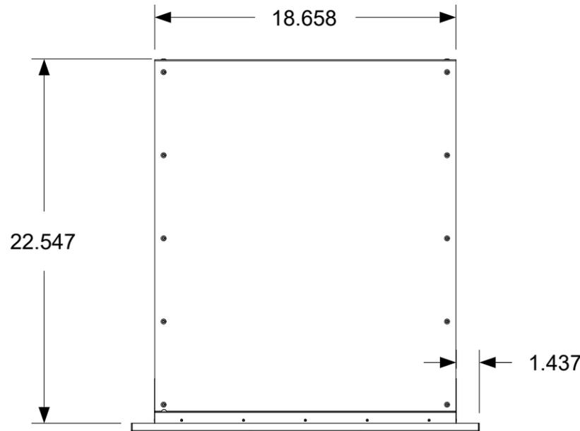
Dimensions shown are the actual physical dimensions. Additional clearances to the cabinetry are dependent on the tolerances of the cut-out. The suggested cut-out dimensions are listed in the chart below but these dimensions can be reduced if the tolerances are controlled. Please refer to the product manual for installation instructions.
