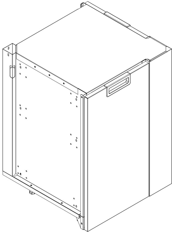
The cabinet provides a 90 degree connection point between other Infinite components. The two doors provide access to a large storage area; there are no drawer options available.
