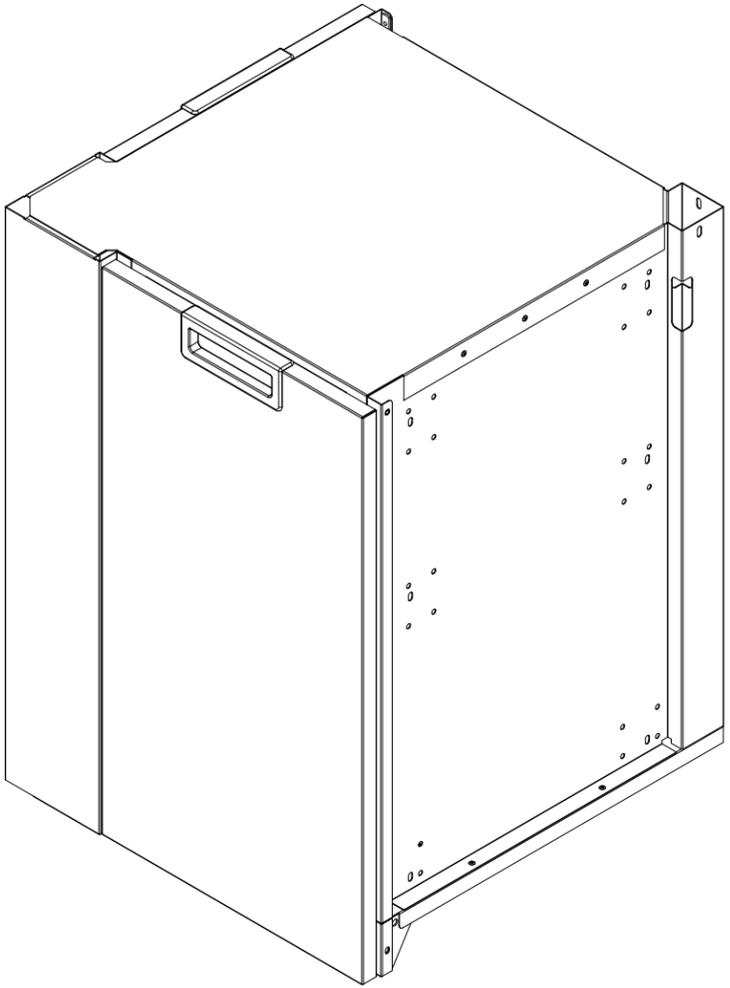
Door shown with lefthand mounting option. Door hardware can be switched to a righthand mount.
