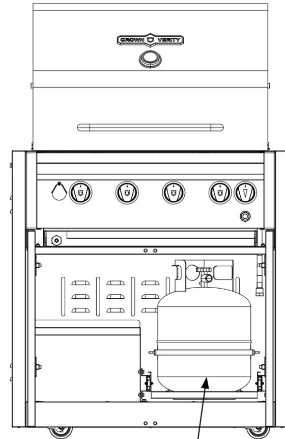
For LP applications that are not connected to a bulk supply, a pull-out propane drawer is factory installed along with a hose and regulator assembly for a 20 lbs. propane tank (not supplied). A shelf is also installed to prevent the storage of a second propane tank per the residential standard for outdoor cooking appliances ANSI Z21.58-2018 and CSA 1.6-2018
