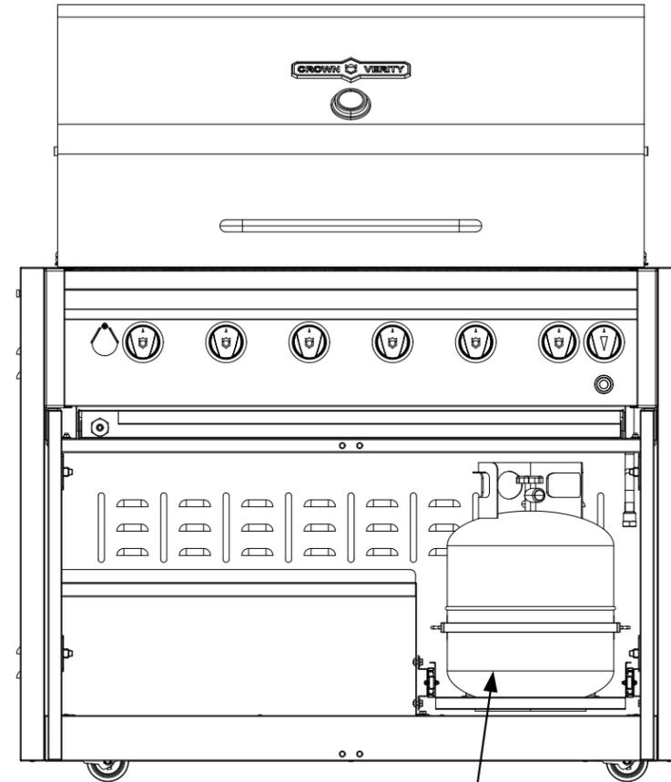
For LP applications that are not connected to a bulk supply, a pull-out propane drawer is factory installed along with a hose and regulator assembly for a 20 lbs. propane tank (not supplied). A shelf is also installed to prevent the storage of a second propane tank per the residential standard for outdoor cooking appliances ANSI Z21.58-2018 and CSA 1.6-2018
