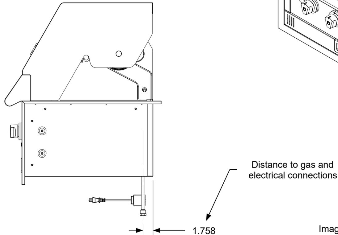
The dimensions shown are the actual physical dimensions of the grill. Additional clearances to cabinetry are dependent on the tolerances of the cut-out. The suggested cut-out dimensions are listed in the chart below but these dimensions can be reduced if the tolerances are controlled.
